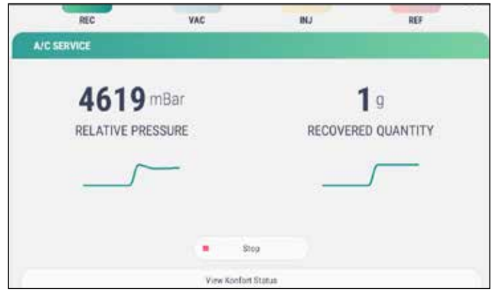
«Recovery» phase: the screen highlights the time remaining until the refrigerant recovery operation is complete.
